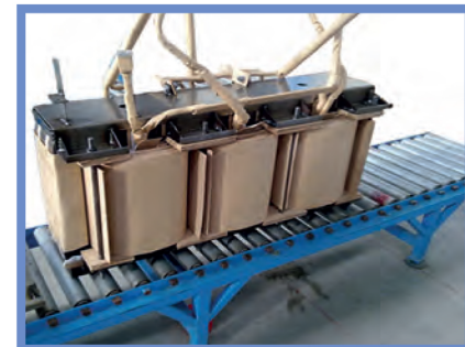
Core Coil Assembly of AMDT
