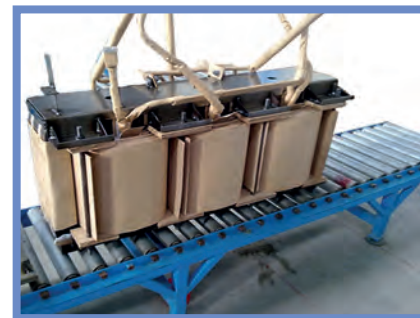
Core Coil Assembly of AMDT
